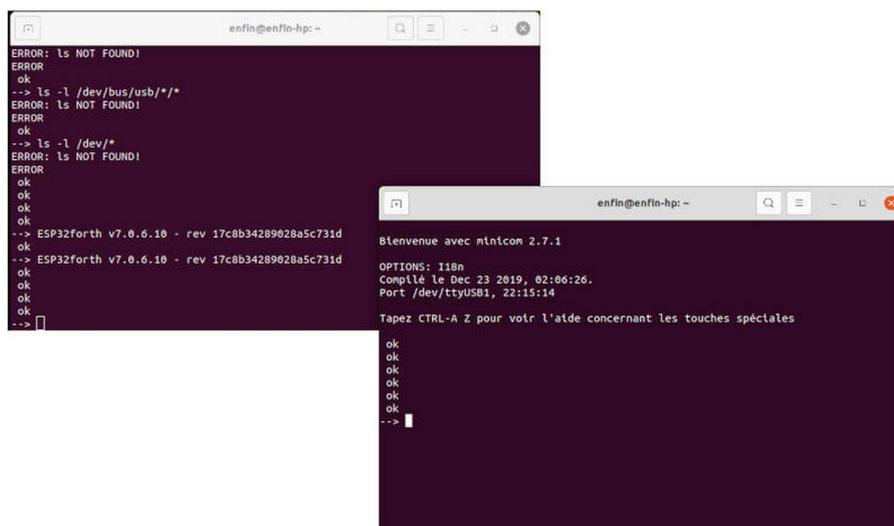
The image shows two terminal windows. The left window shows the user attempting to list USB devices and directories, receiving 'ERROR: ls NOT FOUND!' messages. The right window shows the Minicom interface with a welcome message and instructions to press CTRL-A Z for help.
