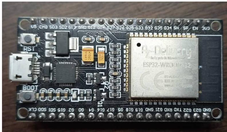
Figure 1: position des E/S GPIO
